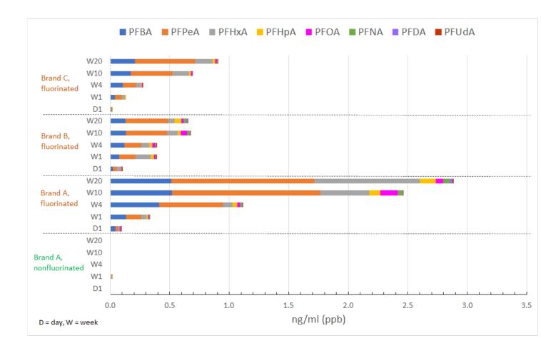
**Figure 2**. Amount of PFAS in methanol stored in fluorinated HDPE containers over time. A nonfluorinated container was used as comparison. The amount of PFAS leached into methanol from one brand of container, although elevated, showed a random pattern of amount leached over time. Individual containers (250 ml size) were used for each time point and the variations among different container replicates may have contributed to the difference in the leached amount for this brand.
